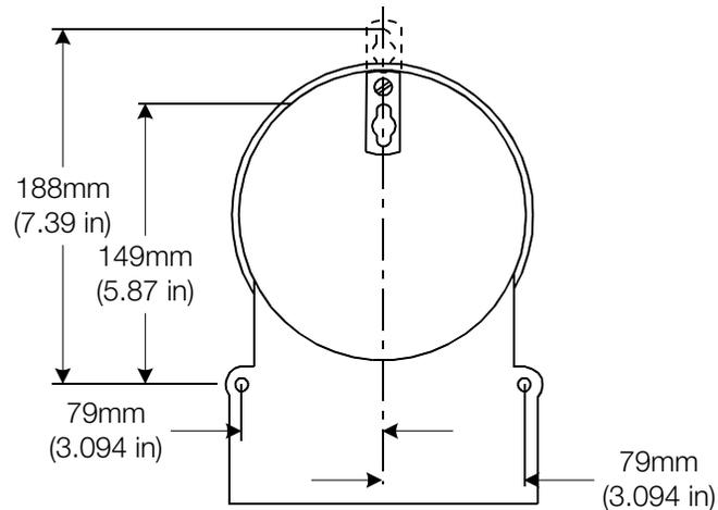
Figure 5–3. Mounting diagram for A–base meters
