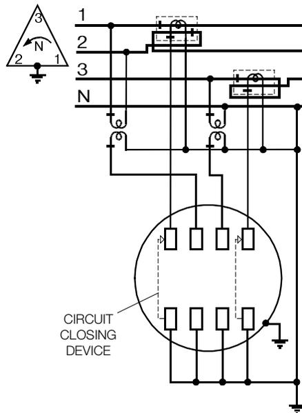
Figure D-27. Form 35S, 3-phase, 4-wire delta, 2 CTs, 2 VTs
