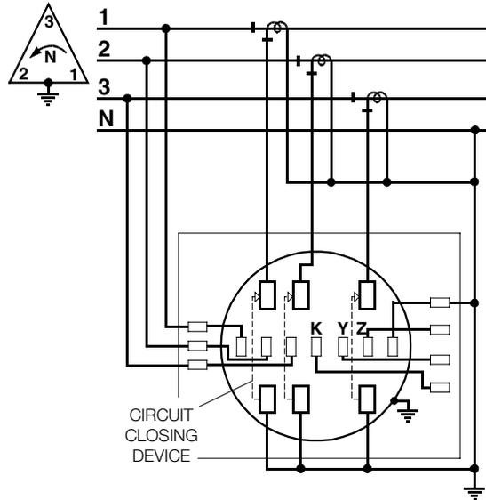
Figure D-6. Form 9S, 3-phase, 4-wire delta, 3 CTs, 0 VTs
