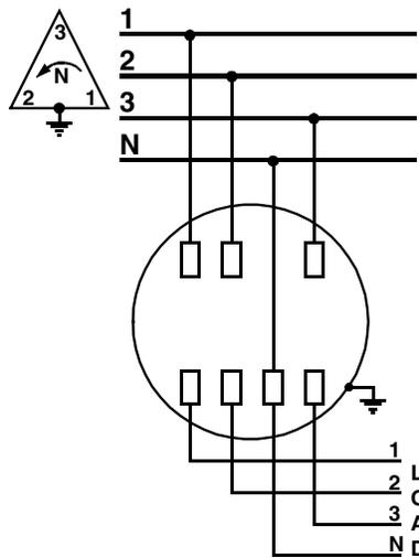
Figure D-19. Form 16S, 3-phase, 4-wire delta, self contained
