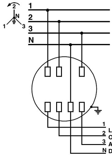
Figure D-20. Form 16S, 3-phase, 4-wire wye, self contained
