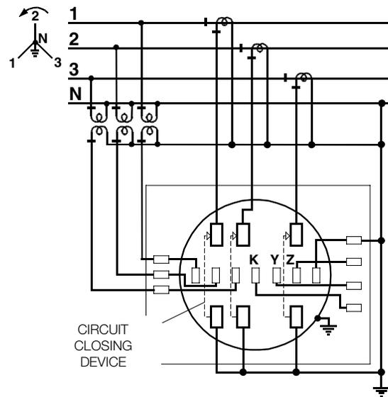
Figure D-7. Form 9S, 3-phase, 4-wire wye, 3 CTs, 0 or 3 VTs
