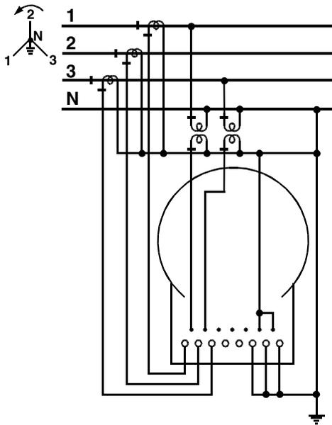
Figure D-29. Form 36A, 3-phase, 4-wire wye, 3 CTs, 0 or 2 VTs
