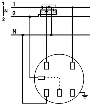
Figure D-4. Form 3S, 1-phase, 3-wire, transformer rated
