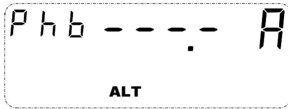
Figure 3-5. Instrumentation phase B current in process
