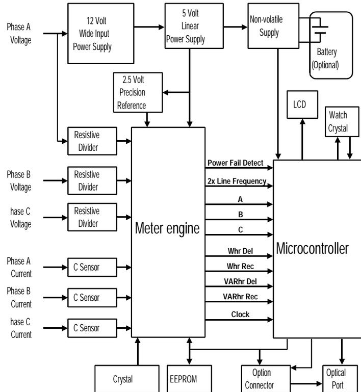
Figure 2–2. Circuit board block diagram
