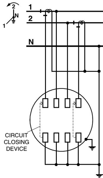
Figure D-25. Form 35S, 2-phase, 3-wire wye, 2 CTs, 0 or 2 VTs
