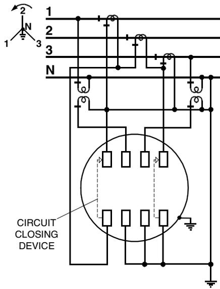
Figure D-28. Form 35S, 3-phase, 4-wire wye, 3 CTs, 0 or 2 VTs
