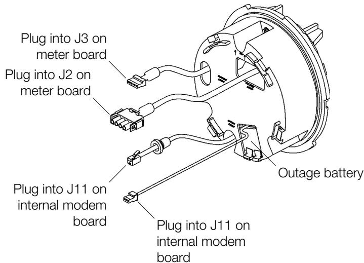
Figure 2–7. Internal modem wiring and outage battery location
