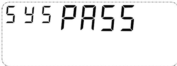
Figure 3-11. System test successful completion
