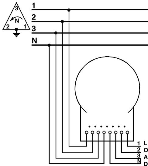
Figure D-17. Form 16A, 3-phase, 4-wire delta, self contained
