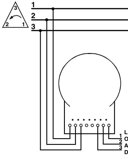
Figure D-15. Form 13A, 3-phase, 3-wire delta, self contained
