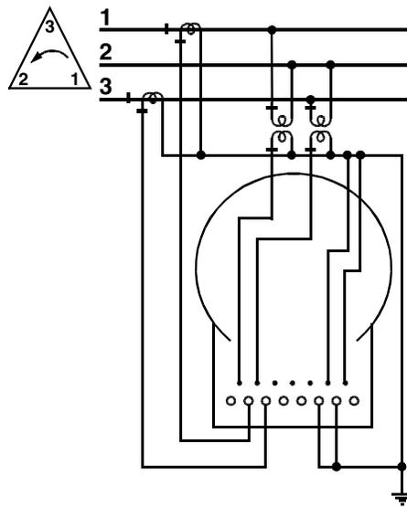
Figure D-22. Form 35A, 3-phase, 3-wire delta, 2 CTs, 0 or 2 VTs
