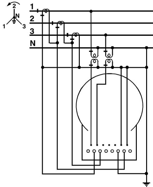
Figure D-24. Form 35A, 3-phase, 4-wire wye, 3 CTs, 0 or 2 VTs
