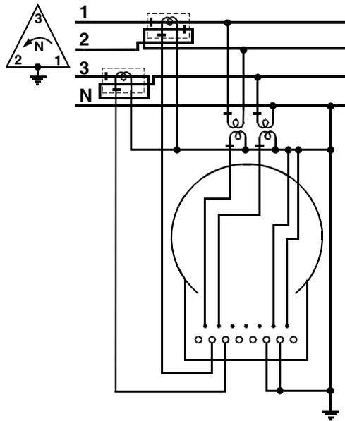
Figure D-23. Form 35A, 3-phase, 4-wire delta, 2 CTs, 2 VTs
