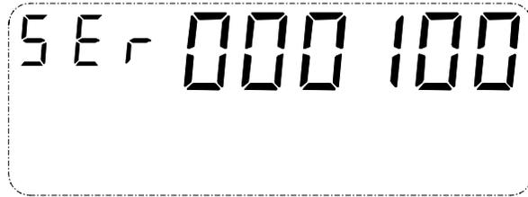
Figure 3-12. System test current service test error
