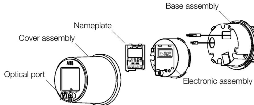
Figure 2–1. Exploded view of the ALPHA Plus meter
