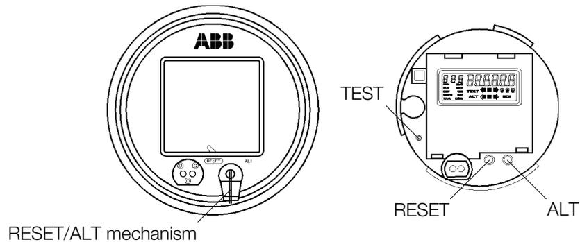
Figure 3-1. Location of push buttons and RESET/ALT mechanism
