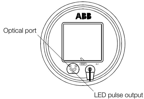
Figure 6–1. Location of the Meter Optical Port and LED Pulse Output
