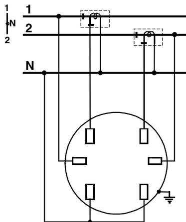
Figure D-5. Form 4S, 1-phase, 3-wire, transformer rated
