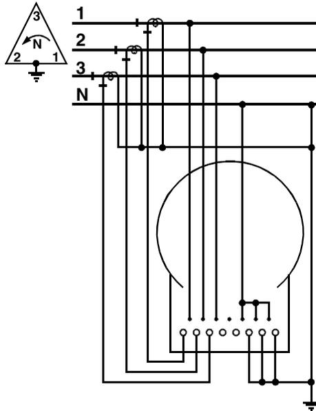
Figure D-8. Form 10A, 3-phase, 4-wire delta, 3 CTs, 0 VTs
