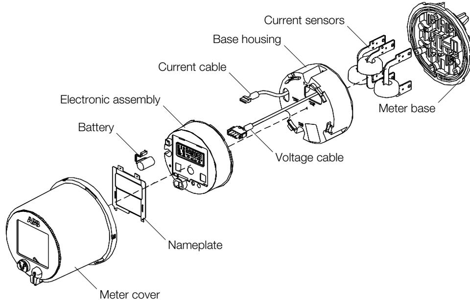
Figure 7-1. Disassembled ALPHA Plus meter
