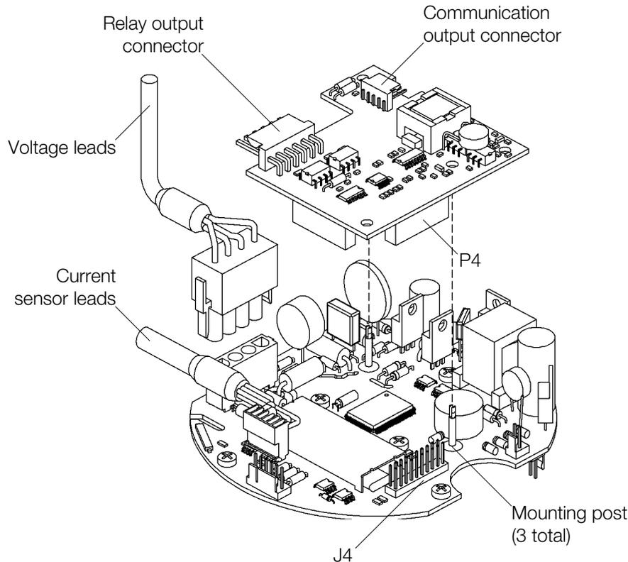
Figure 2–8. ALPHA Plus meter with external communications option board (RS232/485 option board with 2 relays shown)
