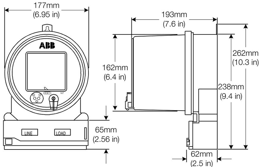
Figure 5-2. Bottom-connected (A-base) meter, front and side view
