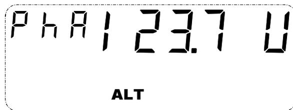
Figure 3–3. Instrumentation phase A voltage
