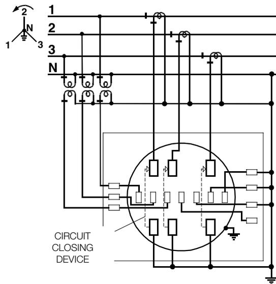
Figure 11. Form 10S, 3-phase, 4-wire wye, 3 CTs, 0 or 3 VTs
