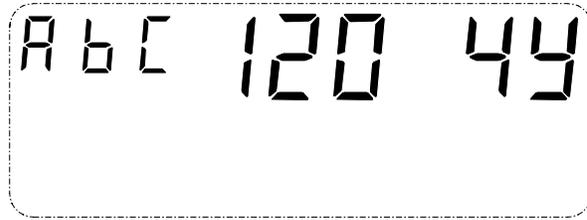
Figure 3-8. System test valid service found
