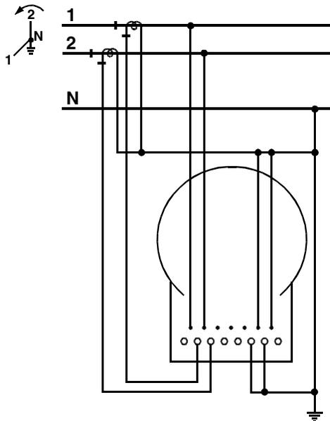
Figure D-21. Form 35A, 2-phase, 3-wire wye, 2 CTs, 0 or 2 VTs
