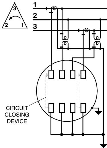
Figure D-26. Form 35S, 3-phase, 3-wire delta, 2 CTs, 0 or 2 VTs
