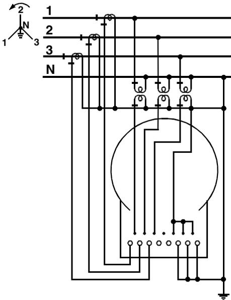
Figure D-9. Form 10A, 3-phase, 4-wire wye, 3 CTs, 0 or 3 VTs
