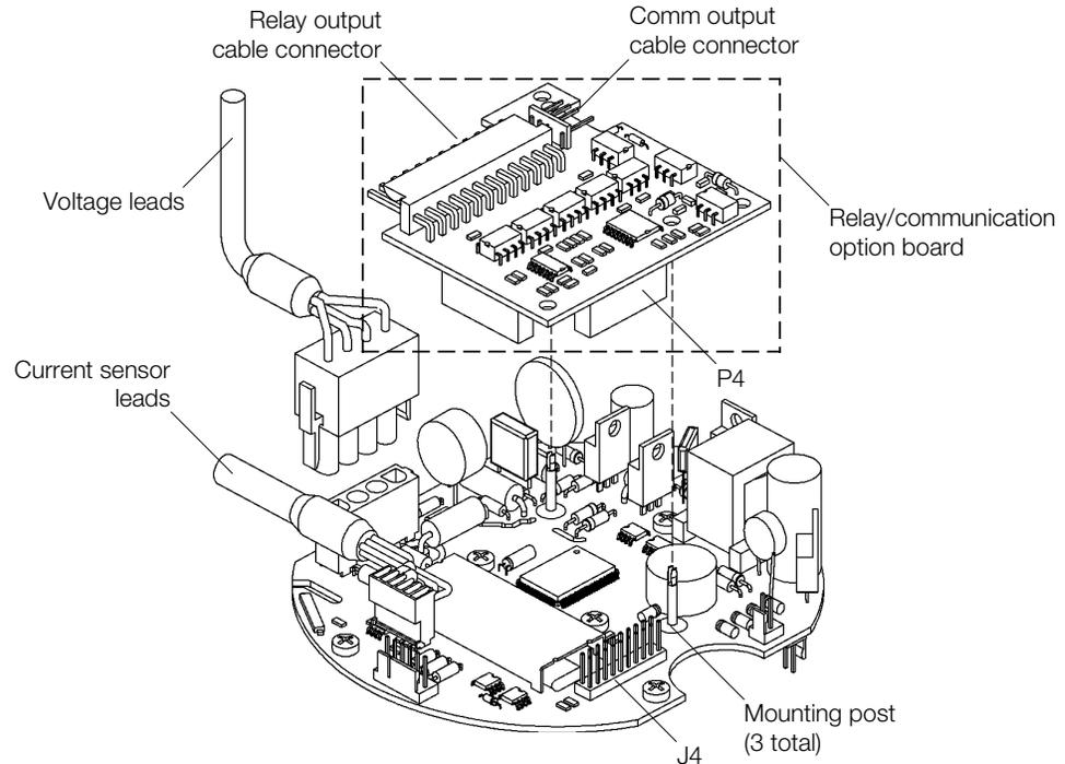
Figure 2-5. ALPHA Plus meter with relay option board
