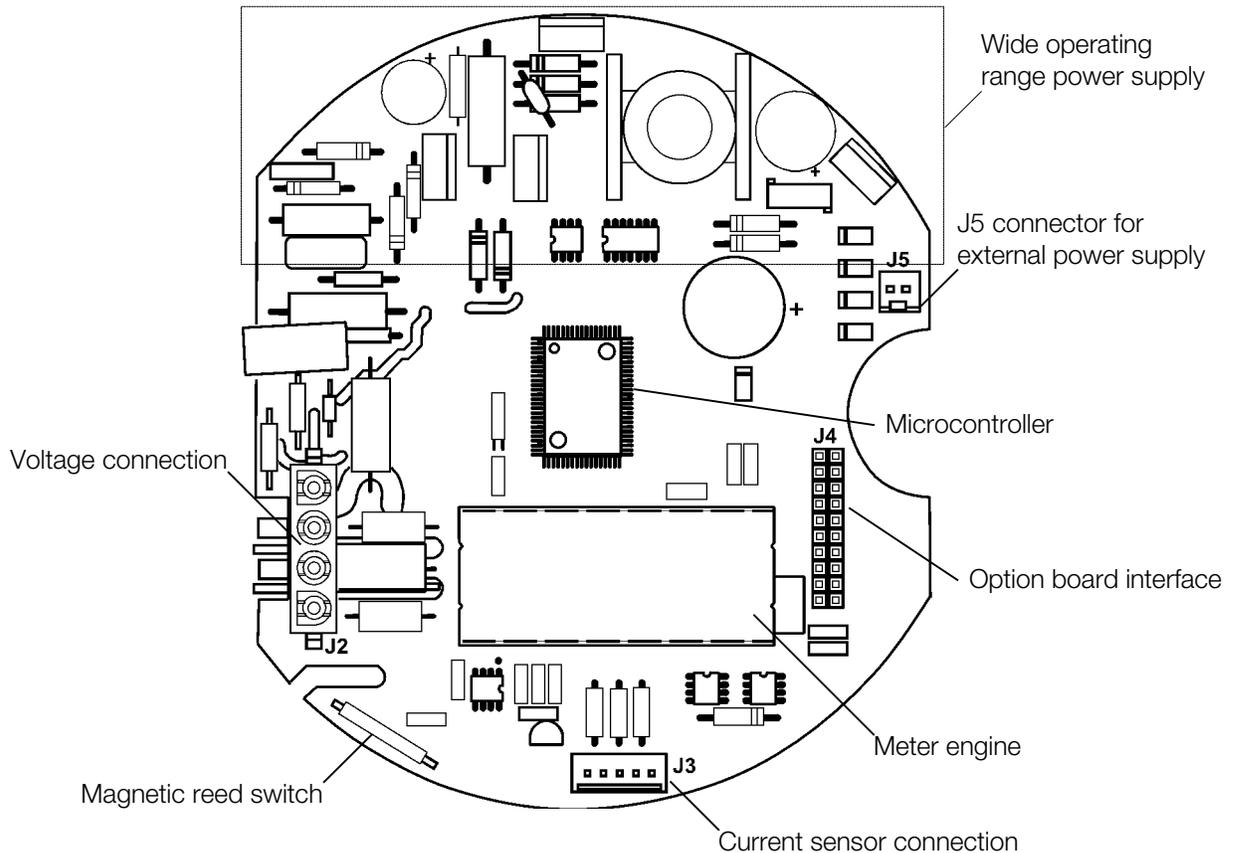
Figure 2-3. ALPHA Plus meter main circuit board
