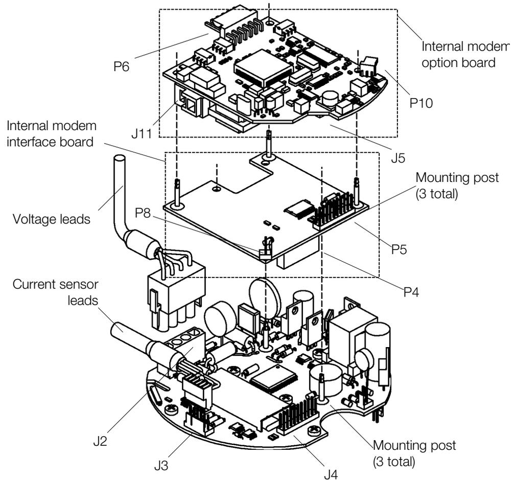
Figure 2–6. ALPHA Plus meter with internal modem (2 relays)
