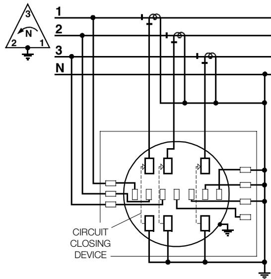
Figure D-10. Form 10S, 3-phase, 4-wire delta, 3 CTs, 0 VTs
