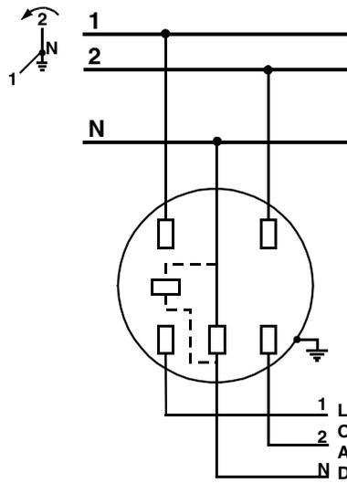
Figure D-12. Form 12S, 2-phase, 3-wire wye, self contained
