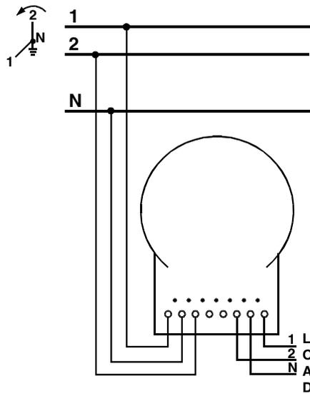
Figure D-14. Form 13A, 2-phase, 3-wire wye, self contained
