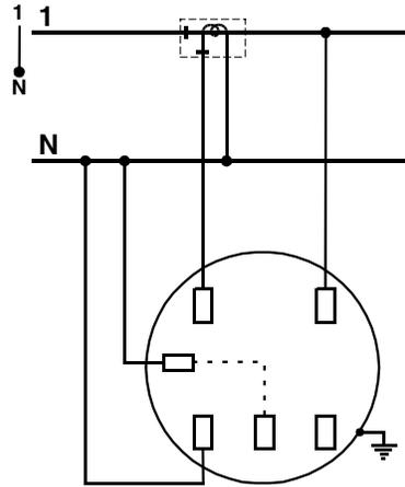
Figure D-3. Form 3S, 1-phase, 2-wire, transformer rated
