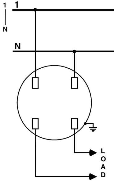
Figure D-1. Form 1S, 1-phase, 2-wire, self contained
