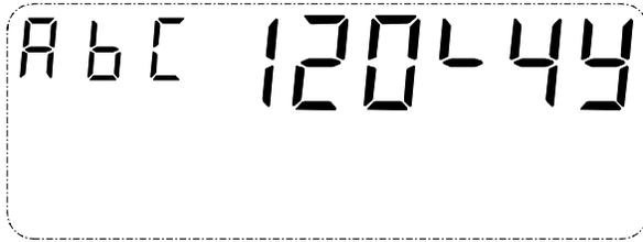
Figure 3-10. System test valid service found and locked
