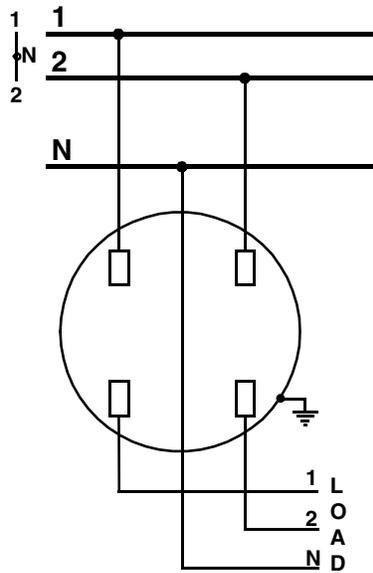
Figure D-2. Form 2S, 1-phase, 3-wire, self contained
