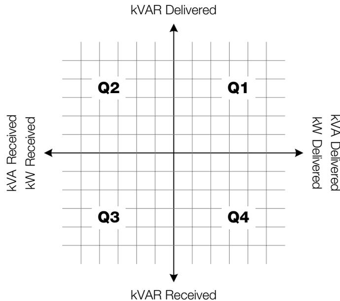
Figure A-1. Four quadrant metering quantity relationships
