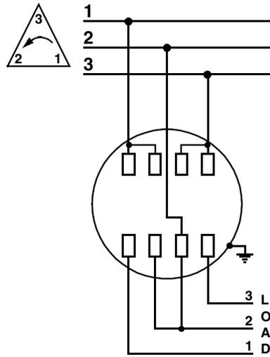
Figure D-16. Form 13S, 3-phase, 3-wire delta, self contained
