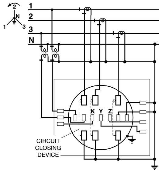
Figure D-30. Form 36S, 3-phase, 4-wire wye, 3 CTs, 0 or 2 VTs
