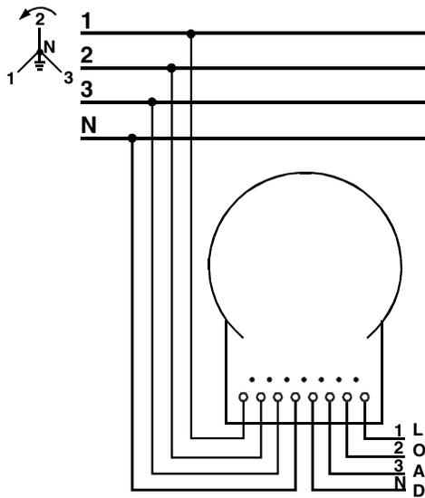
Figure 18. Form 16A, 3-phase, 4-wire wye, self contained
