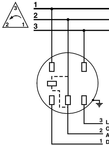
Figure D-13. Form 12S, 3-phase, 3-wire delta, self contained
