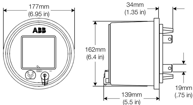
Figure 5-1. Socket-connected (S-base) meter, front and side view
