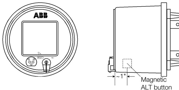
Figure 3-2. Magnetic placement for activating alternate mode
