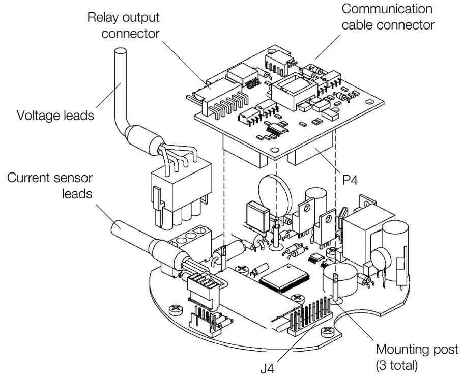
Figure 2–9. ALPHA Plus meter with WAN option board
