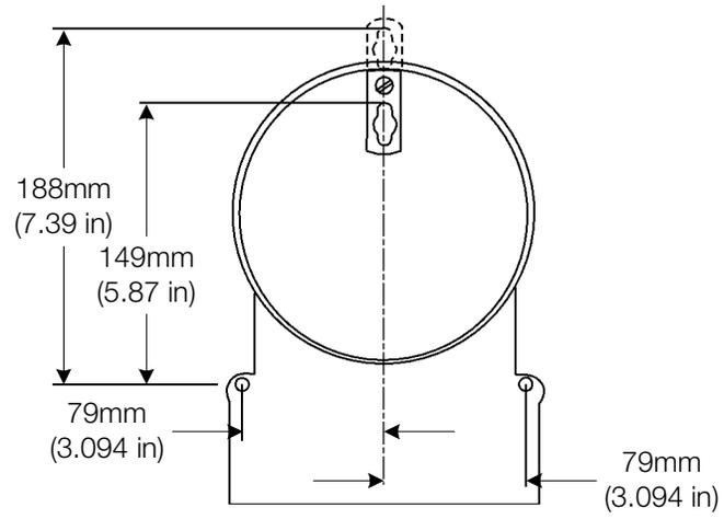
Figure 2-8. A-base meter type and dimensions, back view
