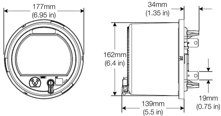
Figure 2-6. S-base meter type and dimensions, front and side view
