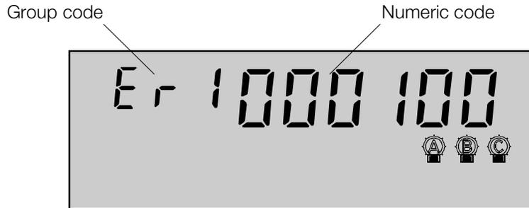
Figure 6-1. Sample error code displayed on the LCD
