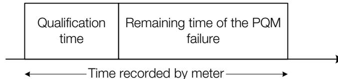
Figure 4-9. Total PQM failure time
