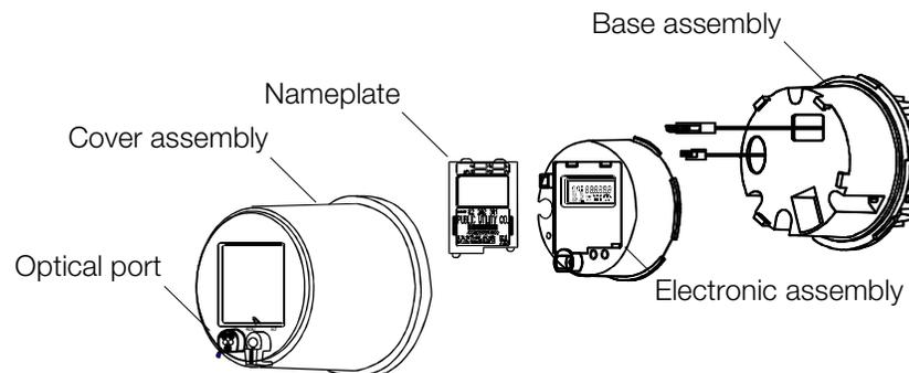
Figure 2-5. Exploded view of the A3 ALPHA meter
