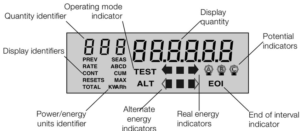
Figure 3-1. Liquid crystal display
