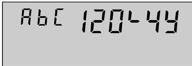
Figure 4-6. Sample display of locked service voltage
