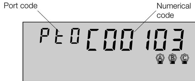
Figure 6-3. Sample communication code displayed on the LCD
