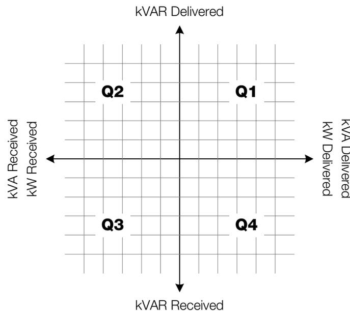
Figure A-1. Four quadrant metering quantity relationships
