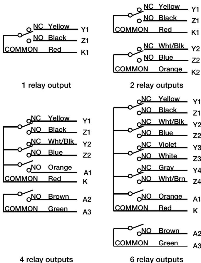
Figure 5-1. Color-coded wiring diagrams for 1, 2, 4, and 6 relays
