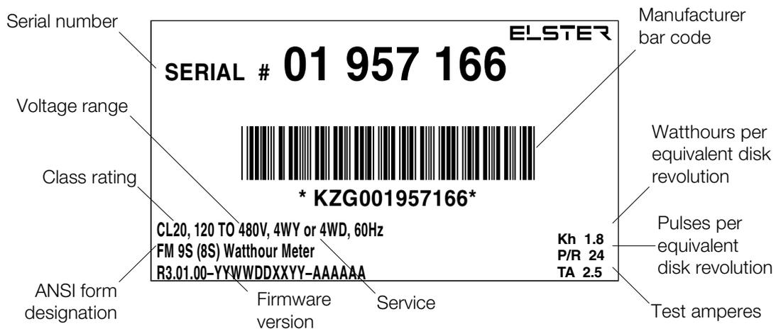
Figure C-5. Lower portion of standard nameplate
