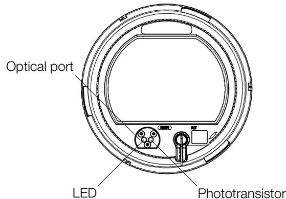
Figure 5-2. Optical port components
