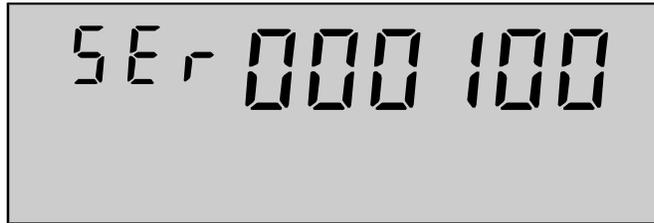
Figure 4-8. Service current test error
