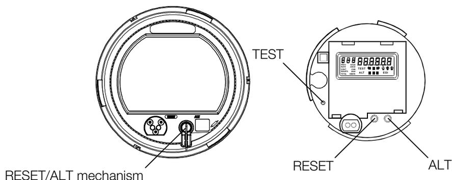
Figure 3-3. Location of push buttons and RESET/ALT mechanism
