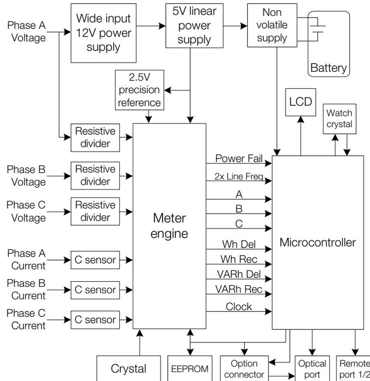
Figure 2-1. Circuit board block diagram
