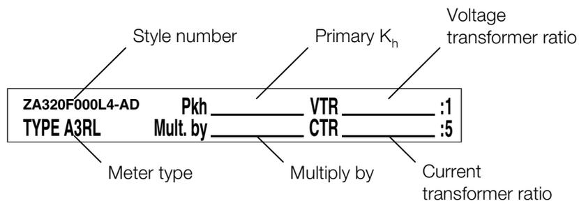
Figure C-2. Top portion of the standard nameplate (transformer rated)
