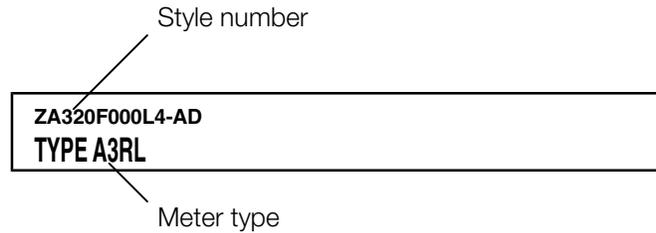
Figure C-3. Top portion of the standard nameplate (self contained)
