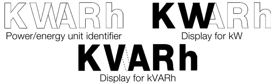
Figure 3-2. Power/energy units identifier
