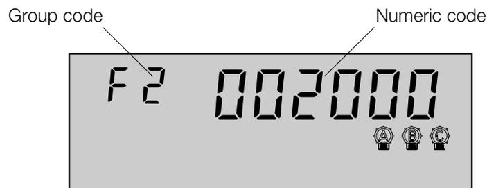
Figure 6-2. Sample warning code displayed on the LCD
