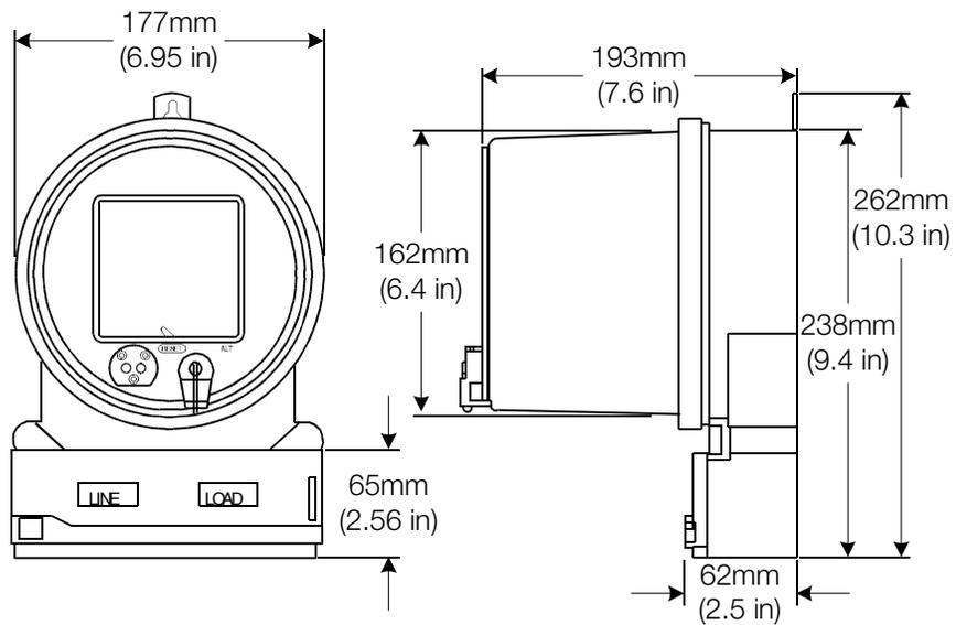
Figure 2-7. A-base meter type and dimensions, front and side view
