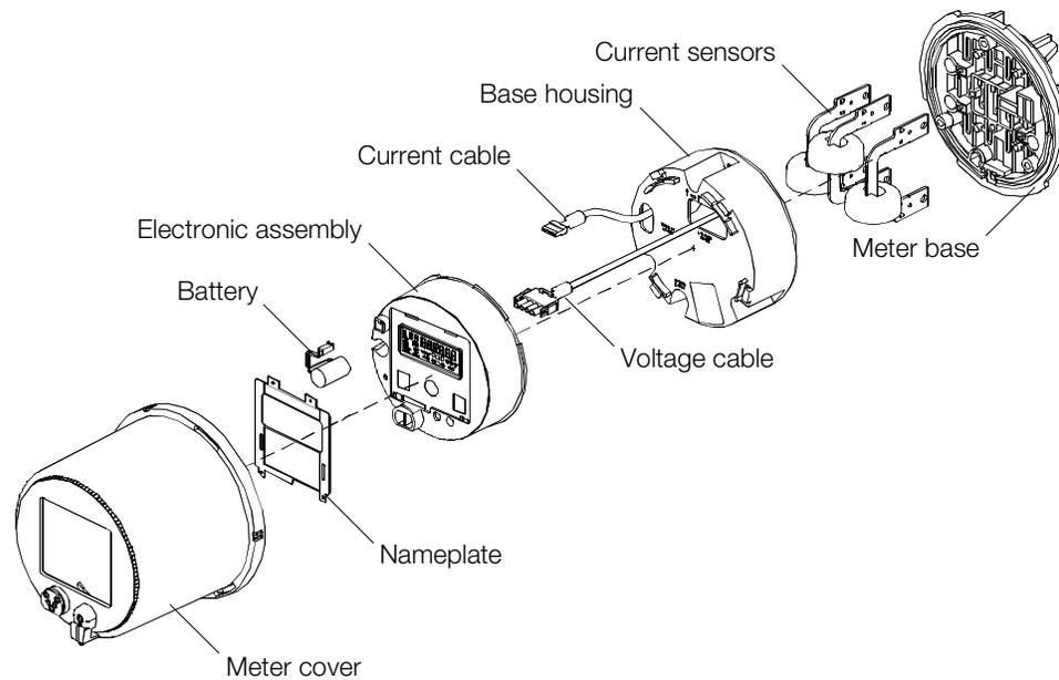
Figure 7-1. Disassembled A3 ALPHA meter
